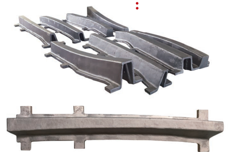
Lay-Up Mandrel for Raked Wing Composite Part
